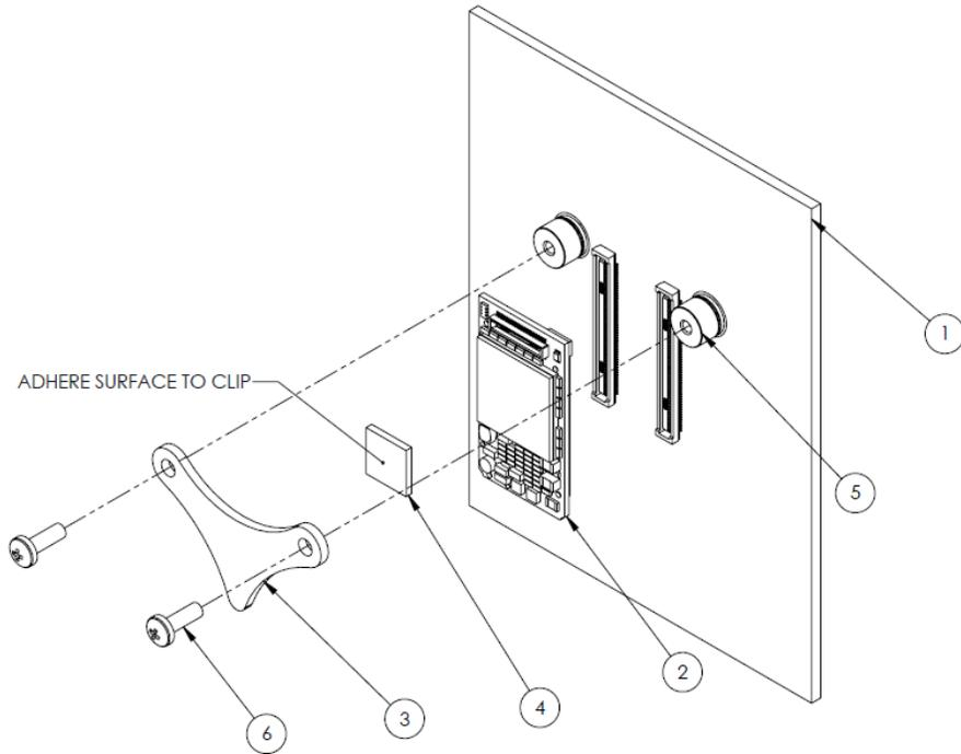
**Figure 6.2: Torpedo SOM Hold-Down Clip Assembly**
