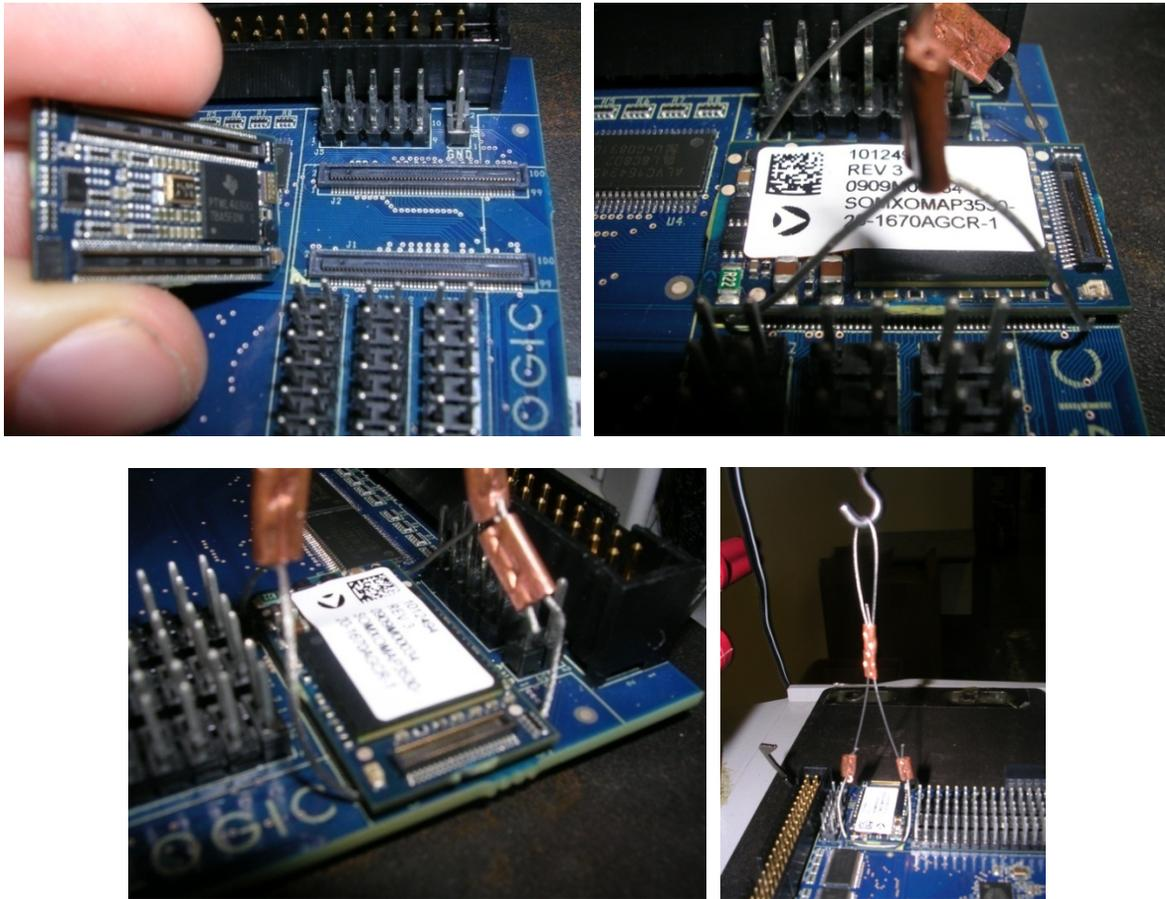
Figure 2.1: Extraction Force Test Harness
