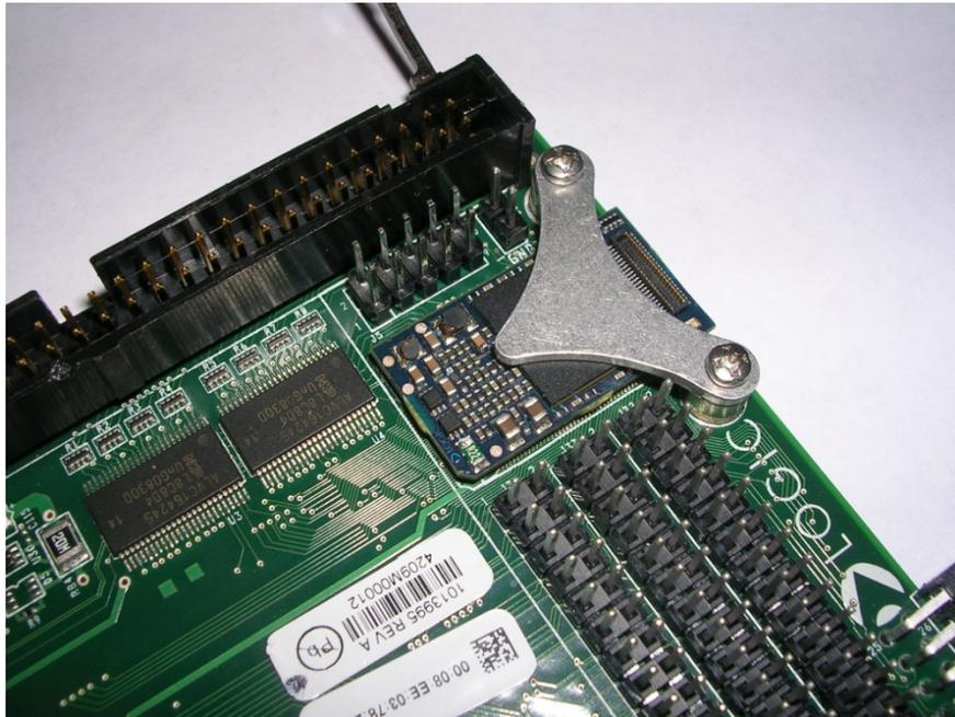
**Figure 6.3: Torpedo SOM Hold-Down Clip**
