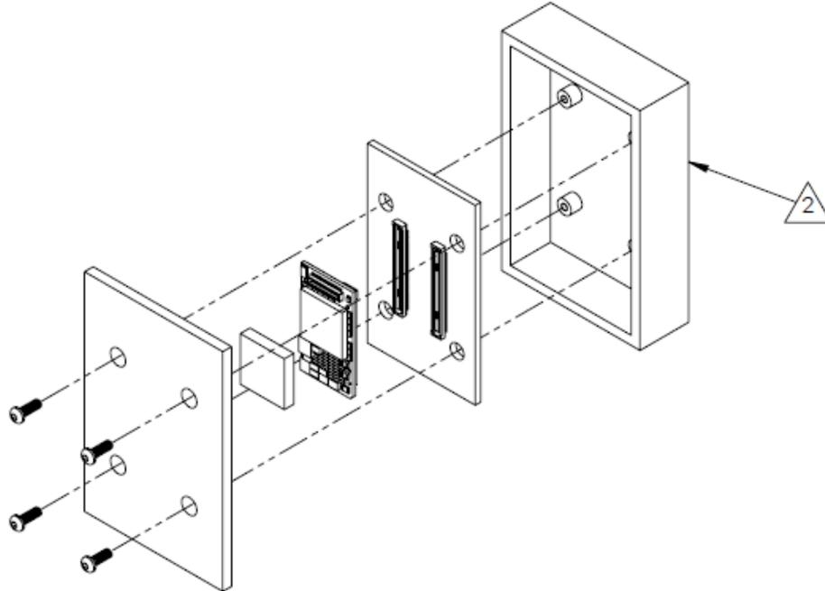
**Figure 6.1: Torpedo In-Housing Retention System Assembly**
