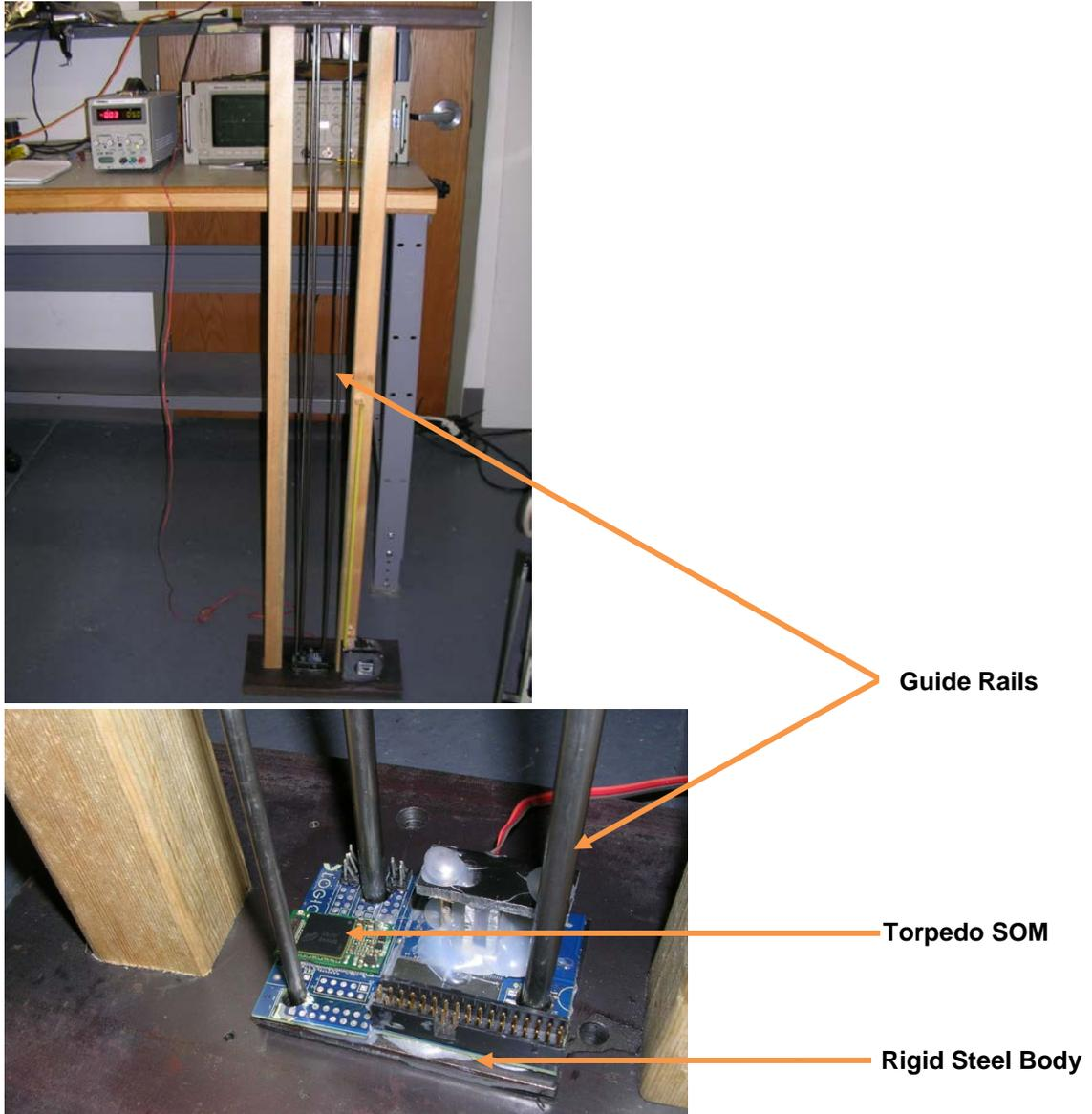
**Figure 4.1: Torpedo Drop Fixture**
