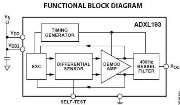
*Figure 4.4: ADXL193 Accelerometer Functional Block Diagram*
