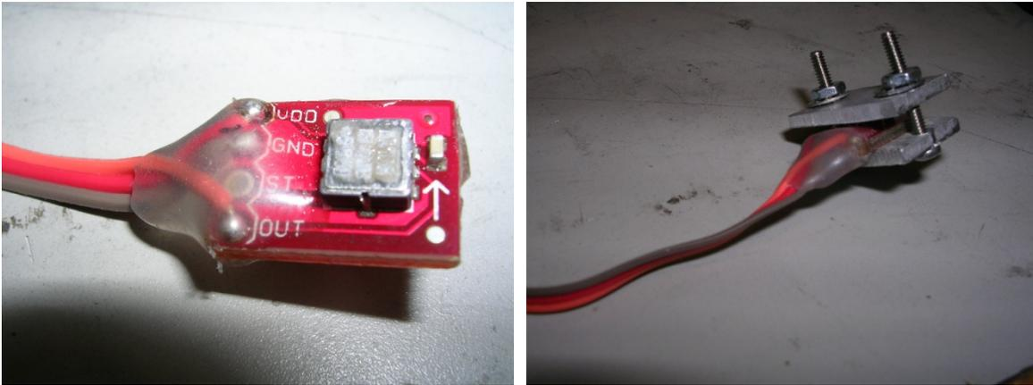
**Figure 4.2: Accelerometer Breakout Board & Vertical Mount**
