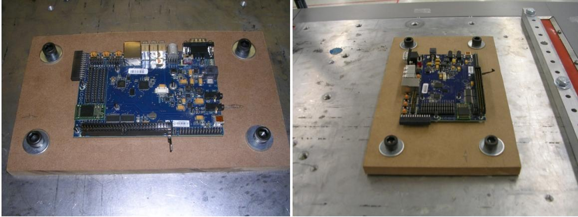
*Figure 3.1: Vibration Test Fixture*
