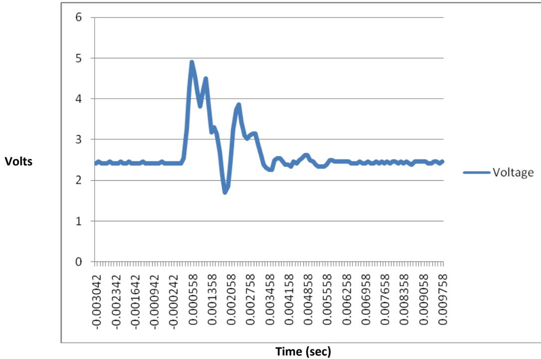
**Figure 4.5: Accelerometer Voltage during Impact as Unit 1 Disconnected**
