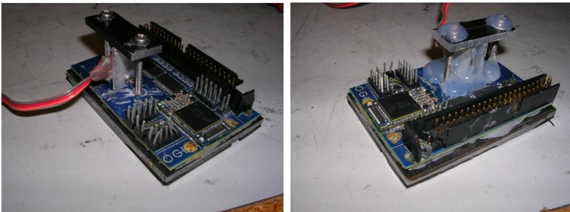
**Figure 4.3: Accelerometer Mounted to Torpedo Carrier Board**
