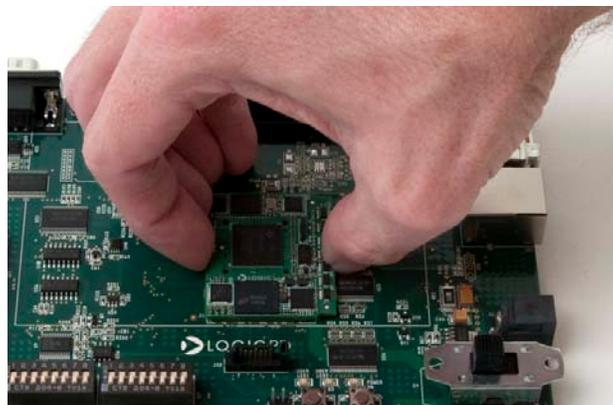
3. To connect the AM1808 SOM-M1, align the SOM over the three board-to-board connectors. Using even pressure, press straight down over the connectors to mate boards. Visually verify that all three connectors have fully mated.
