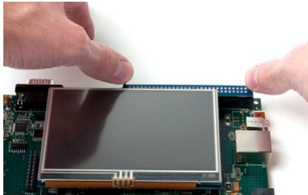
2. Taking care not to bend the PCB, remove the AM1808 SOM-M1 by applying even pressure beneath the PCB edges and pulling up.
