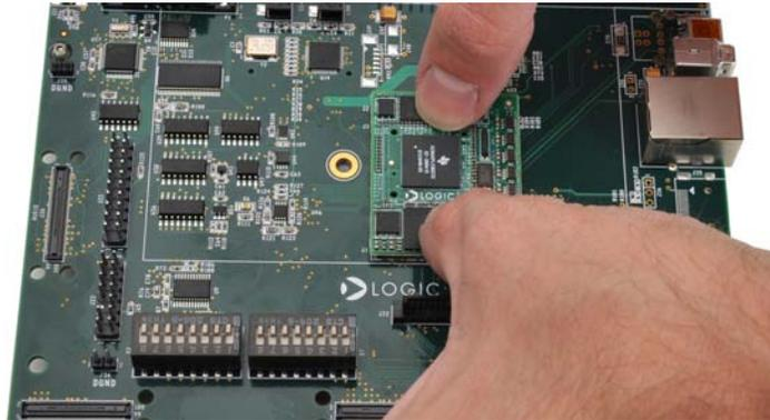
4. Connect the 4.3" LCD by inserting into the baseboard LCD connector and pushing down over the connector until the LCD ejector levers move to a vertical position. **CAUTION:** The solder points on the LCD connector PCB may be sharp; use caution when connecting the LCD.
