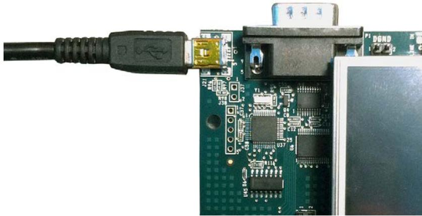
**Figure 2.1: Connection to Emulation USB Port**
