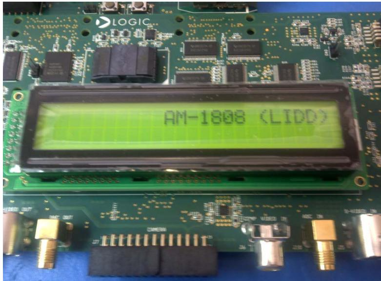
**Figure 3.3: Character LCD Test Display Image**
