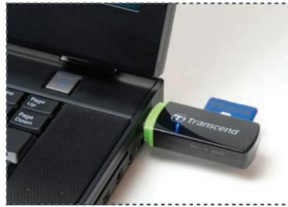
**10** Remove SD card and insert it into included USB SD card reader; connect USB SD card reader to host PC
