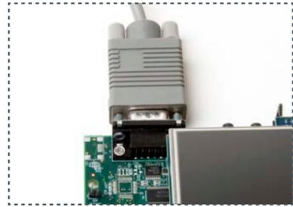
**9** Power off kit and connect serial cable to baseboard and host PC
