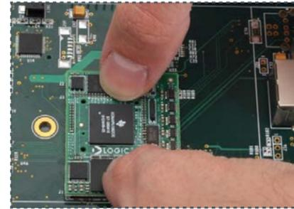
**1** Connect OMAP-L138 SOM (use outline on baseboard for positioning), press straight down over connectors
