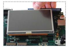
Connect 4.3" LCD, remove protective plastic covering
