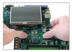
Power off kit and connect UI board to baseboard connectors at center and on the right
