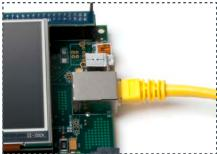
Connect Ethernet cable to baseboard and host PC or router
