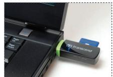
Remove SD card and insert it into included USB SD card reader; connect USB SD card reader to host PC
