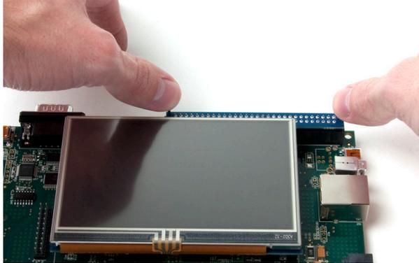
2. Taking care not to bend the PCB, remove the OMAP-L138 SOM-M1 by applying even pressure beneath the PCB edges and pulling up. Set aside OMAP-L138 SOM-M1.
