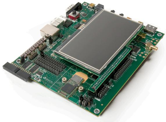
**ZOOM DM3730 TORPEDO DEVELOPMENT KIT WITH INCLUDED DM3730 TORPEDO + WIRELESS SOM & 4.3" WQVGA LCD**
