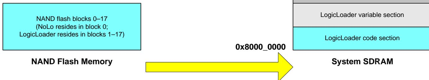
**Figure 1.3: LogicLoader RAM Execution Environment**
