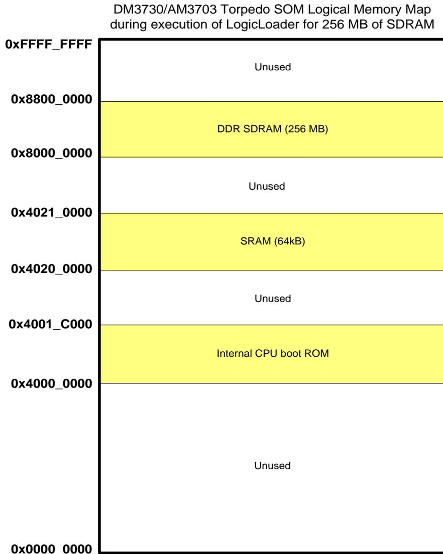
Figure 1.1: DM3730/AM3703 Torpedo SOM Hardware Memory Map
