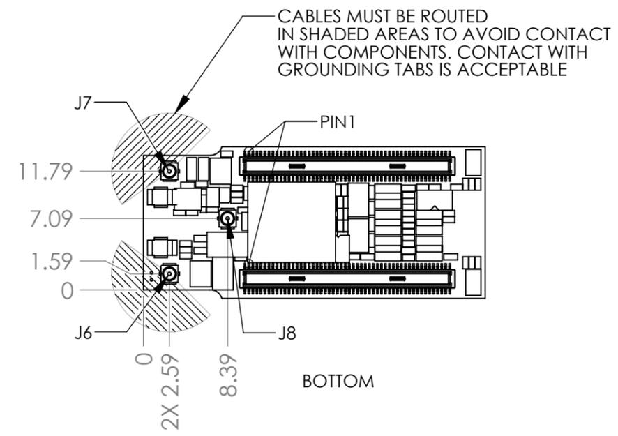
DIMENSIONING AND TOLERANCING TO BE INTERPRETED PER ASME Y14.5-2009
